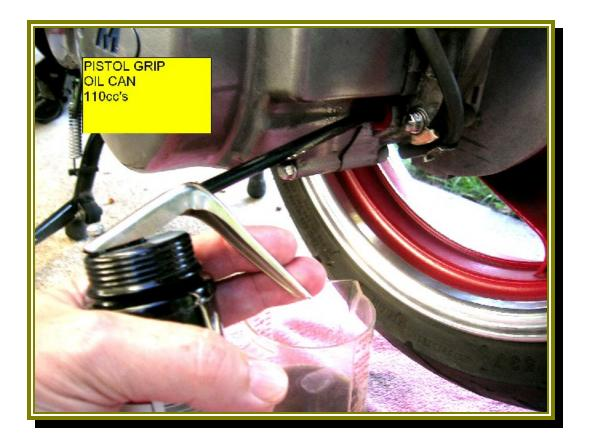
Insert the tube of the oil gun toward the rear of the oil box and squirt the oil gently into the box. Don't squirt so fast that the oil doesn't have time to flow into the box. Once you have emptied the can, replace the fill screw. Wipe everything down and observe for leaks. Take a short ride and observe for leaks again.
